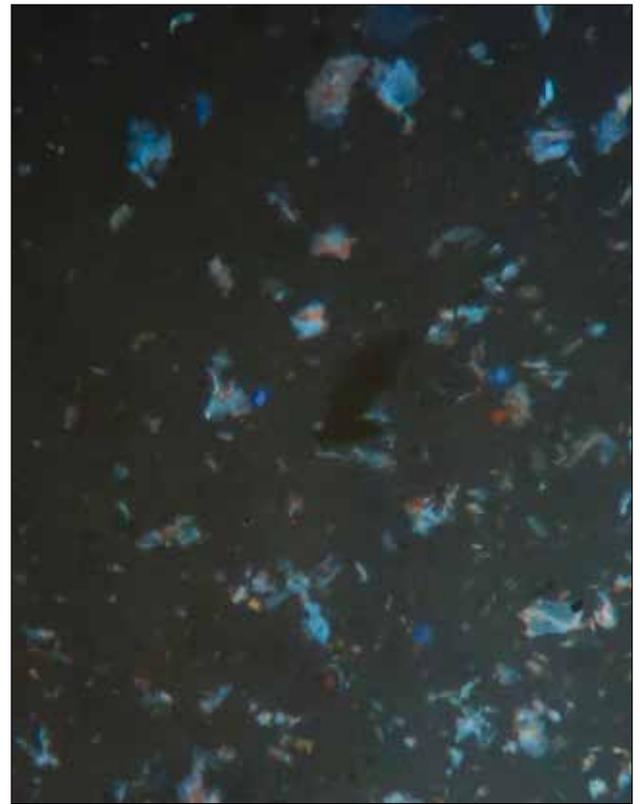
Plate 2. Dispersion of PS524 viewed in plane polarised light x400.
