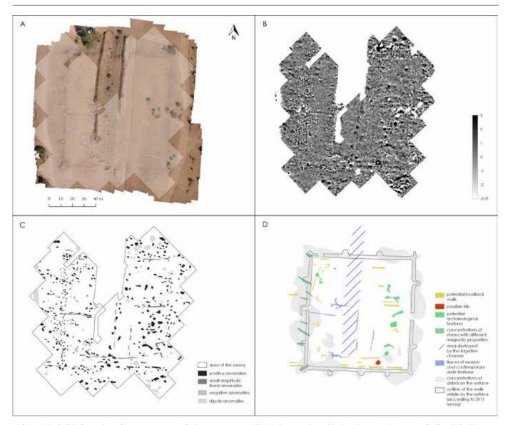
Plate 9. Hosh el-Kah, geophysical survey: A – area of the survey (prepared by M. Drzewiecki and R. Ryndziewicz), B – grayscale plot of the FM265 data, r, dynamics: -3/+3 nT (prepared by R. Ryndziewicz), C – classification of geophysical anomalies (prepared by R. Ryndziewicz), D – archaeological interpretation of the magnetometer data (prepared by R. Ryndziewicz).
