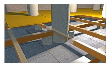
Figure 7. Sanam Abu Dom. Chamber 6 in the Treasury, hypothetical arrangement of girders resting on the dwarf columns, the joists and floorboards, with detail of the relationship adjacent to the central row of roof-supporting columns.
