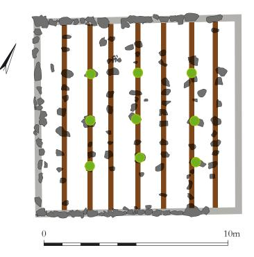
Figure 4. Site P4 – plan of the remains with a suggested reconstruction of the raised floor timbers and location of the timber posts supporting the roof - scale 1:150.
