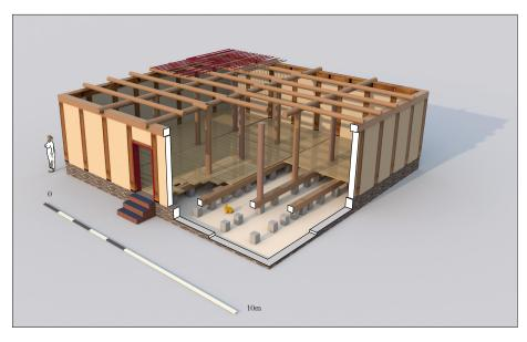
Figure 5. Site P4 - hypothetical reconstruction of the building with its raised floor and timber framed construction.
