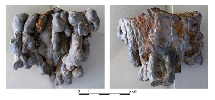
Figure 7. View of the upper and lower faces of a tapped slag (MWSS1C2.01) (cl. N. Dieudonné-Glad, HeRMA, Université de Poitiers).
