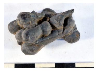
Figure 17. Cord-like slag with only one broken end (MWS2002.13); (cl. N. Dieudonné-Glad, HeRMA, Université de Poitiers).
