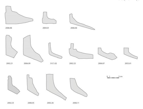
Figure 10. Cross section of a slag formed after a vertical flow of the viscous material in Area 2.
