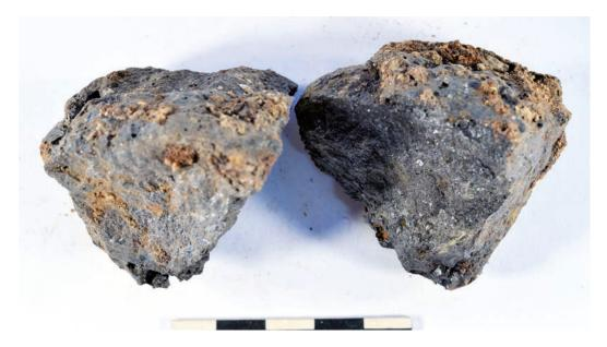
Figure 11. View of the break of a solid slag (MWS2002.05) (cl. N. Dieudonné-Glad, HeRMA, Université de Poitiers).
