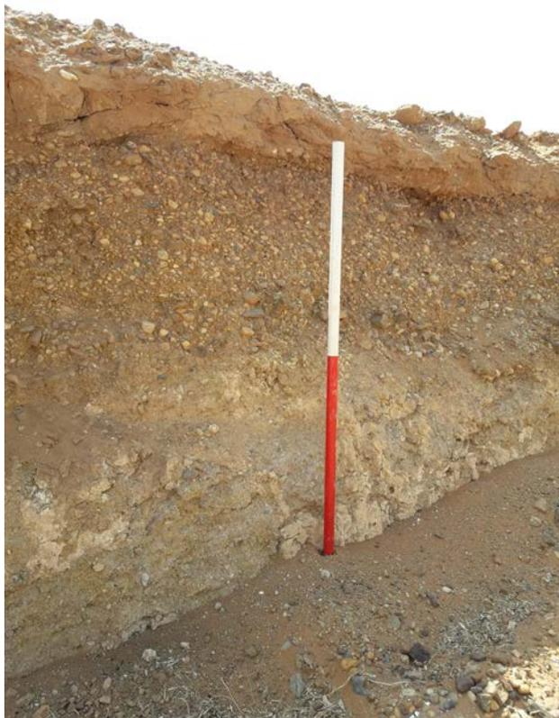
Figure 5. Trench showing the various geological layers: 1) fine sandy limestone – surface layer; 2) gravel layer (concrete) mixed with a little fine sand; 3) hard calcareous layer (© Fakhri Hassan Abdallah, NCAM).
