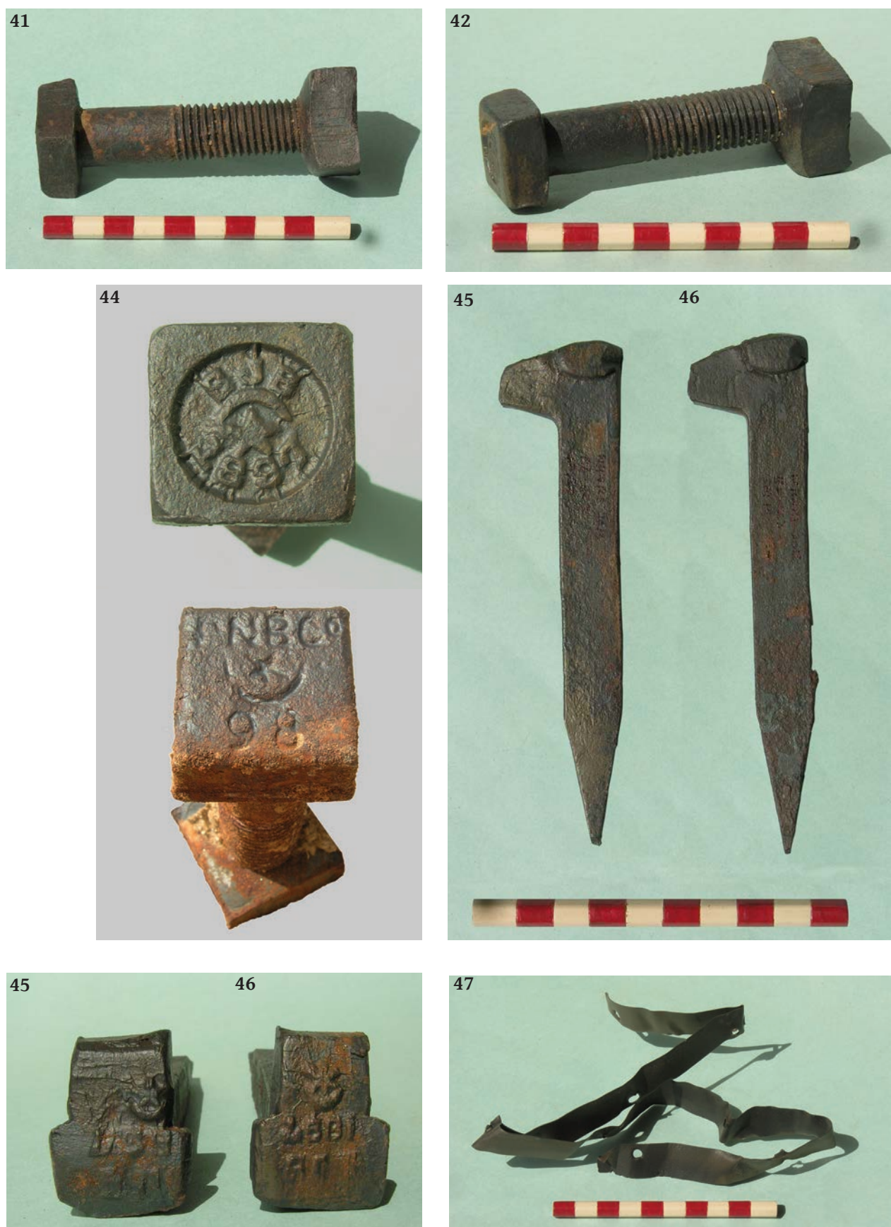
Figure 67. Fishplate bolts, doghead spikes and banding iron. Catalogue nos 41-42, 44-47.
