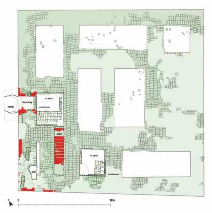
Figure 4. Plan of building H 3000 indicating the foyer H 3004 and the main entrance in the west, staircase H 3002 and casemate H 3003 (scale 1:200).
