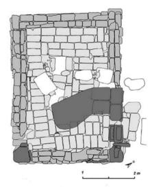
Figure 7. Ground plan of talatat chapel B 700-sub 2 excavated March, 2008. Drawn by Manja Wetendorf-Lavall (scale 1:100). The dark blocks are Kushite or stones reused in Kushite times; the irregular mass in the center is the large natural boulder with a New Kingdom inscription on its rear face.
