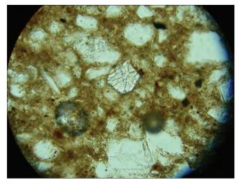
Colour plate XLV. 'Kaolinitic-Nile mix" petrofabric (sample #5), plane-polarized light, field width 0.5 mm. with colourless amphibole (actinolite?) in the centre.
