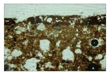
Colour plate XLIII. Red-clay slip on "Kaolinitic-Nile mix" petrofabric (sample #4), plane-polarized light, field width 1mm.
