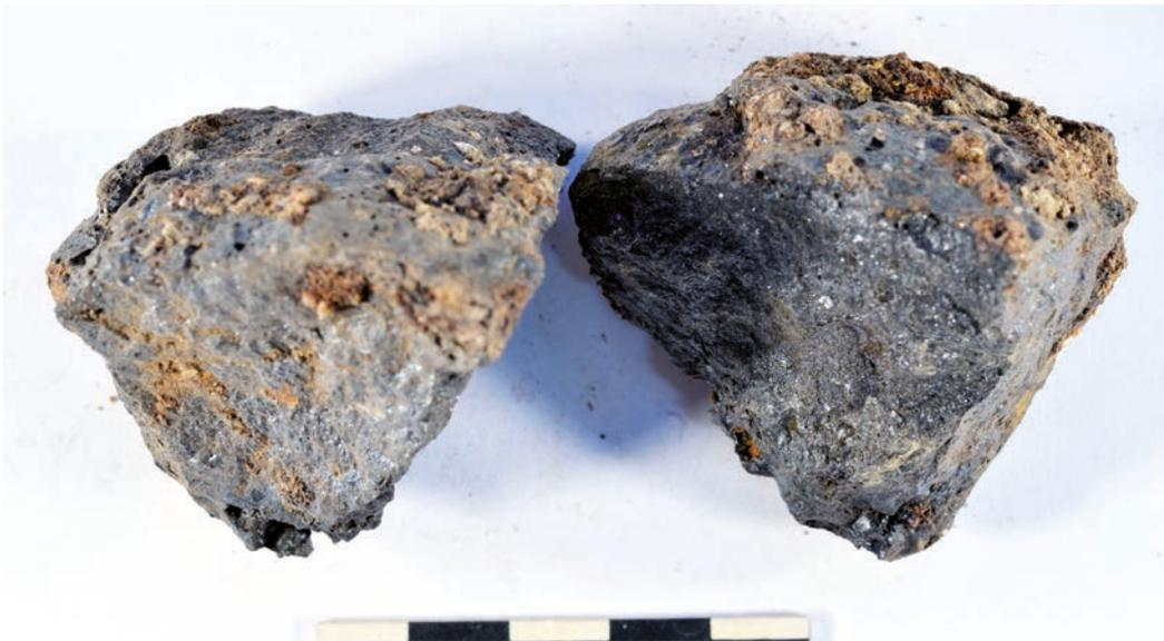
Figure 11. View of the break of a solid slag (MWS2002.05) (cl. N. Dieudonné-Glad, HeRMA, Université de Poitiers).
