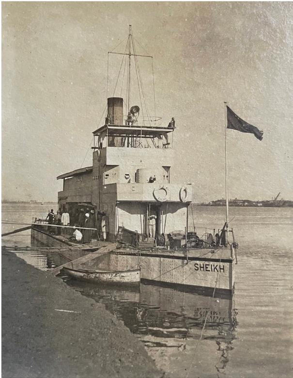
Figure 2. The *Sheikh* moored on the Nile c. 1917. The two Maxim guns and 12-pounder 12-hundredweight guns are clearly visible along with the searchlight. The vessel was in similar condition until 1925 (photo courtesy of J. Anderson).
