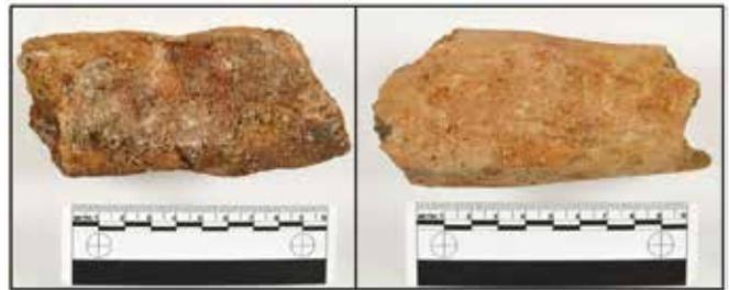
Plate 2. A comparison between a roughly made tuyère (left) and a finely made tapered tuyère (right).
