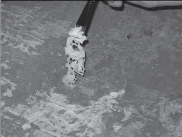
Plate 18. Polyurethane traces are all that was left of the facing.
