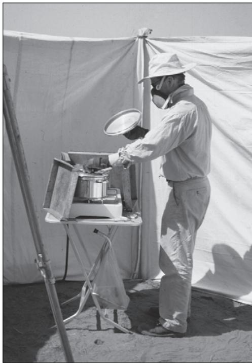
*Plate 2. David Singleton heating CDD and petroleum spirit in a double boiler.*
