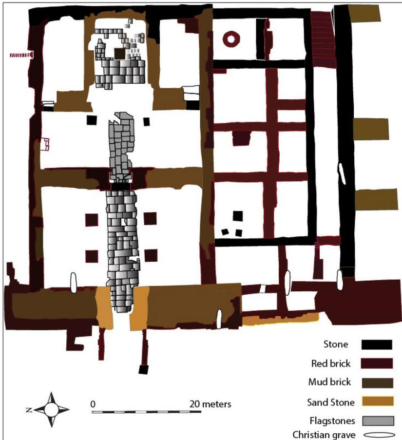
Figure 2. Coloured top level plan of the temple and adjacent rooms showing building materials used.
