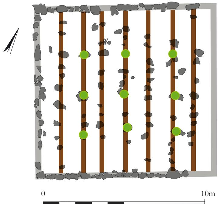
Figure 4. Site P4 – plan of the remains with a suggested reconstruction of the raised floor timbers and location of the timber posts supporting the roof - scale 1:150.
