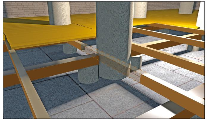
Figure 7. Sanam Abu Dom. Chamber 6 in the Treasury, hypothetical arrangement of girders resting on the dwarf columns, the joists and floorboards, with detail of the relationship adjacent to the central row of roof-supporting columns.
