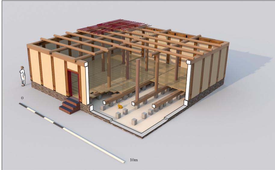
Figure 5. Site P4 - hypothetical reconstruction of the building with its raised floor and timber framed construction.
