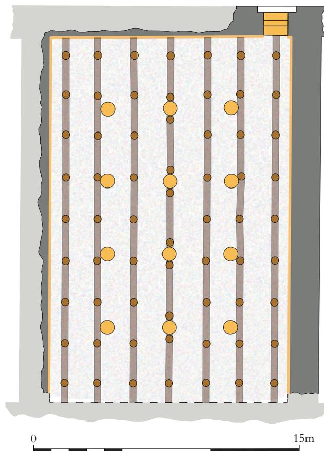
Figure 6. Sanam Abu Dom. Chamber 6 in the Treasury, suggested arrangement of timber girders to support the joists of the raised floor - scale 1:200 (base plan: after Griffith 1922, pl. L).
