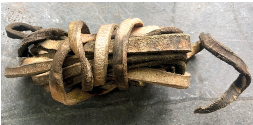
Figure 2. Rawhide strapping – made from the outer edge of a sheet of cattle rawhide.
