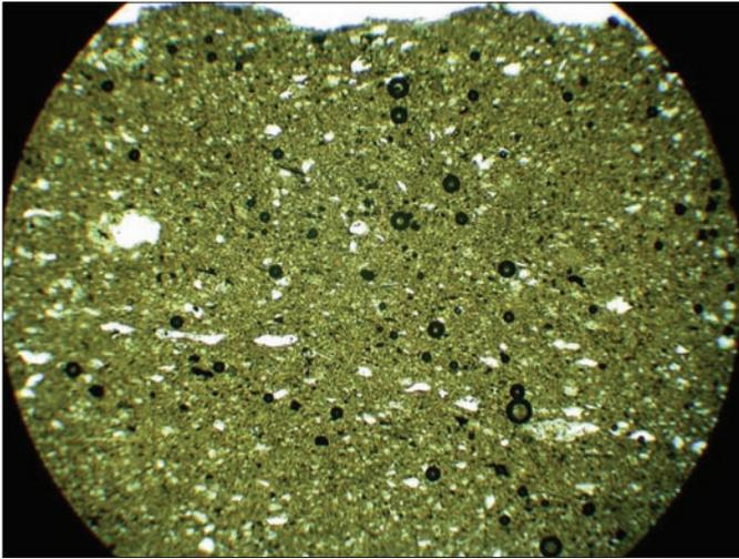
*Colour plate XL. "Meroe Kaolinitic" petrofabric (sample #1), plane-polarized light, field width 3mm.*
