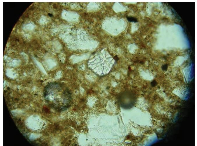
*Colour plate XLV. "Kaolinitic-Nile mix" petrofabric (sample #5), plane-polarized light, field width 0.5 mm. with colourless amphibole (actinolite?) in the centre.*
