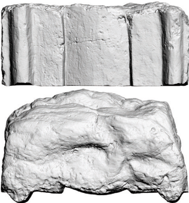
Plate 12. Scan of the portico block (381), Front and top view. Size: width 826mm; height 370mm; depth 503mm.
