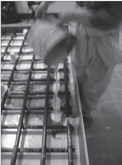
Plate 15. Foamed epoxy resin was poured into the mould.
