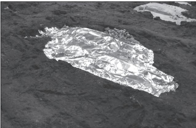
*Plate 12. Holes were filled with vermiculite granules and sealed with aluminium foil tape.*
