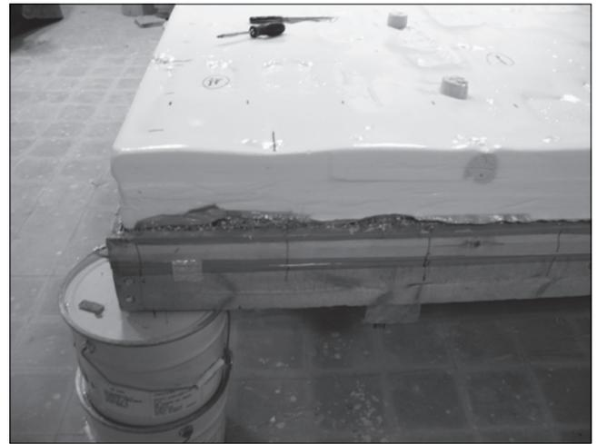
Plate 16. When the foam had hardened the mould was removed.
