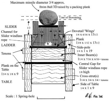
Figure 4. Cross-section of ballista slider from Vitruvius' description, with ovoid Ibrim Ball 3D raised by a packing plank.
