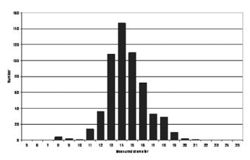
Figure 2. Bar-graph 1, showing the distribution of the measured diameters (7.5-20.5cm; average: 14.3cm) of the 569 ballista balls; 147 are between 13.5 and 14.5cm (Barnard).
